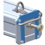
Step5e: Reinstall the latch, and make sure it is seated on the bushings in the end cap.
